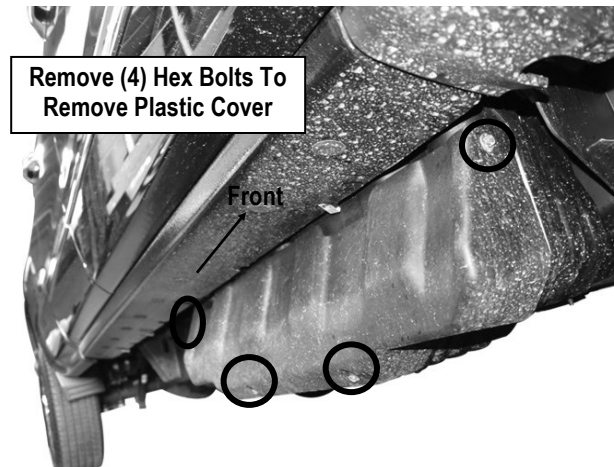
(Fig 10A) 2017-Up 2500/3500 Models Passenger Side Pictured (With DEF Plastic Tank Cover)
