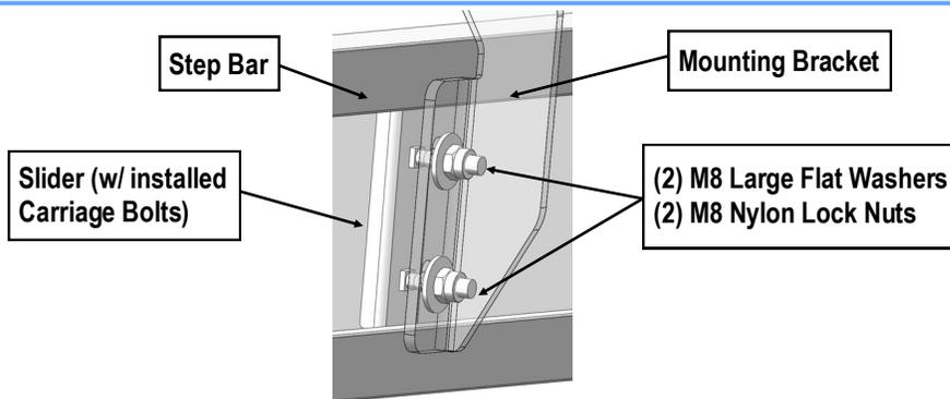
**(Fig 7) Step Bar Installation**
