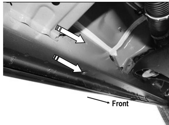
(Fig 3) Passenger 2nd Mounting Bracket Location
