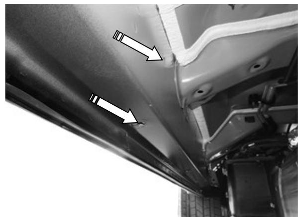
(Fig 4) Passenger 3rd Mounting Bracket Location
