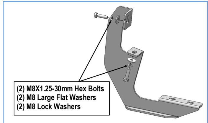
(Fig 2) Passenger Front Mounting Bracket Installation
