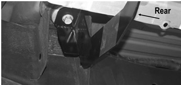
(Fig 8) Passenger Rear Mounting Bracket Installed
