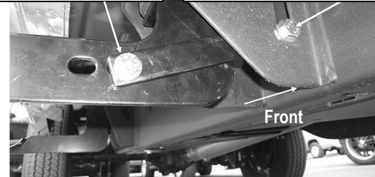
(Fig 6) Passenger Center Bracket Installed (1500 Models)
