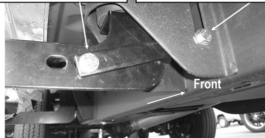
(Fig 6) Passenger Center Bracket Installed (1500 Models)
