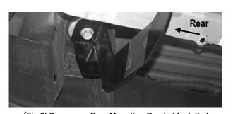
(Fig 9) Passenger Rear Mounting Bracket Installed
