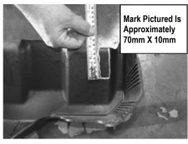
(Fig 14) 2017-Up Passenger Side DEF Cover Marked For Trimming
