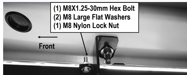
(Fig 21) Attach Passenger Rear Mounting Bracket (the 3rd one) to Pinch Weld
