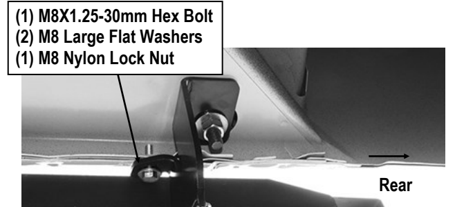
(Fig 22) Attach Passenger Rear Mounting Bracket (The Last One) to Pinch Weld
