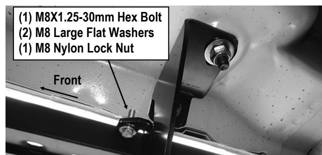
(Fig 20) Attach Passenger Center Mounting Bracket To Pinch Weld
