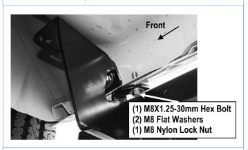
(Fig 16) Attach Passenger Front Mounting Bracket To Pinch Weld
