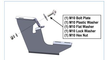
(Fig 3) Driver Front Mounting Bracket (DFM) Installation
