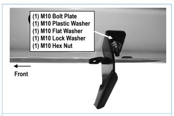
(Fig 15) Passenger Side Rear Mounting Bracket Installation
