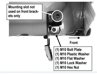
(Fig 4) Driver Front Mounting Bracket (DFM) Installation
