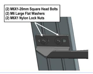
(Fig 7) Running Board Installed Onto Driver Center Mounting
