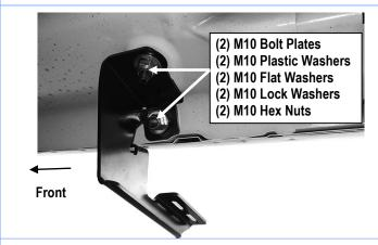
(Fig 13) Passenger Center Mounting Bracket (PCM) Installation
