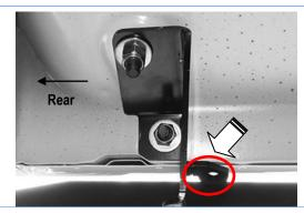
(Fig 8) Drill 5/16" Hole Through Pinch Weld Do Not Drill Too Close To Edge Of Pinch Weld (Driver Side Rear Bracket Pictured)
