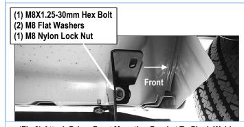
(Fig 9) Attach Driver Front Mounting Bracket To Pinch Weld
