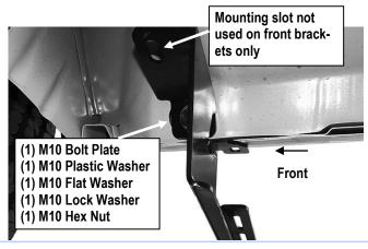
(Fig 12) Passenger Front Mounting Bracket (PFM) Installation
