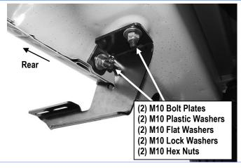
(Fig 5) Driver Rear Mounting Bracket (DRM) Installation
