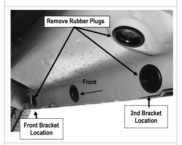
(Fig 11) Passenger Side Front & Center Mounting Bracket Locations
