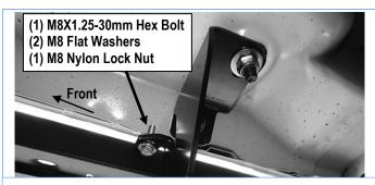
(Fig 17) Attach Passenger Center Mounting Bracket To Pinch Weld
