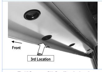
(Fig 14) Passenger Side Rear Mounting Location
