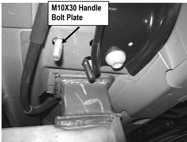
(Fig 6) M10X30 Handle Bolt Plate Installation
