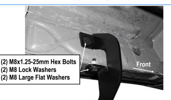
(Fig 6) Driver Front Mounting Bracket Installed
