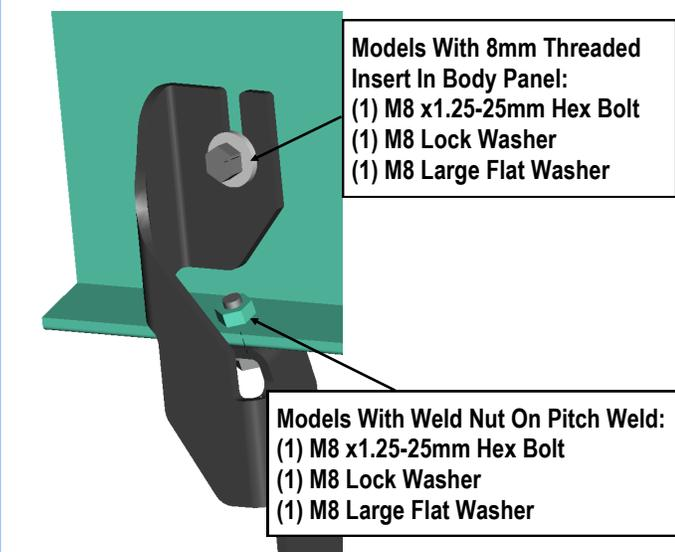
(Fig 18) Passenger Front Mounting Bracket Installation (Weld Nut If Equipped-Also See Fig 2)
