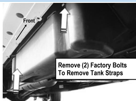
(Fig 11) 07-16 Passenger Side DEF Tank And Cover
