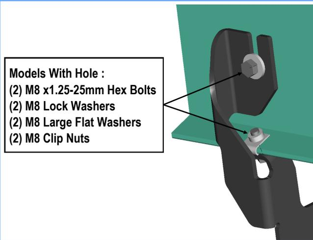
(Fig 17) Passenger Front Mounting Bracket Installed (example)
