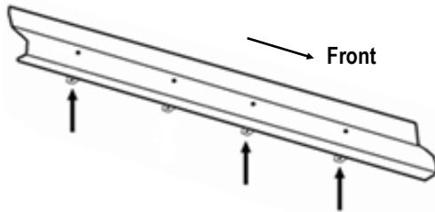
(Fig 1) Driver Side Mounting Locations
