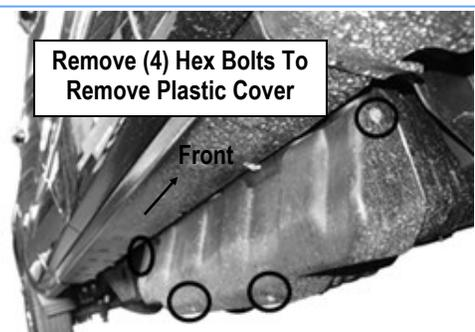
(Fig 10A) 2017-Up Passenger Side Pictured With DEF Plastic Tank Cover.
