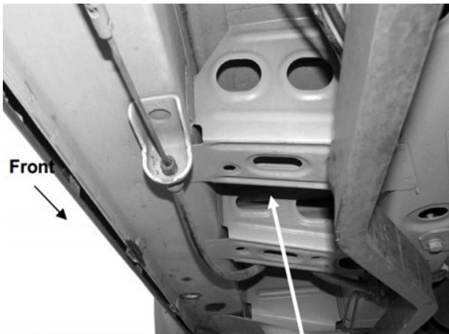
(Fig 5) Driver Center Mounting Bracket Location Pictured
