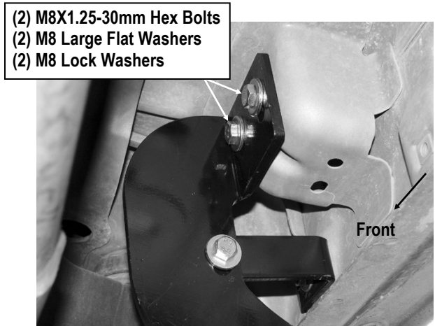
(Fig 3) Passenger Side Front Mounting Bracket Installation (Front View)
