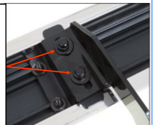
(Fig 7) Step Bar Installed on Bracket Installed (Example)
