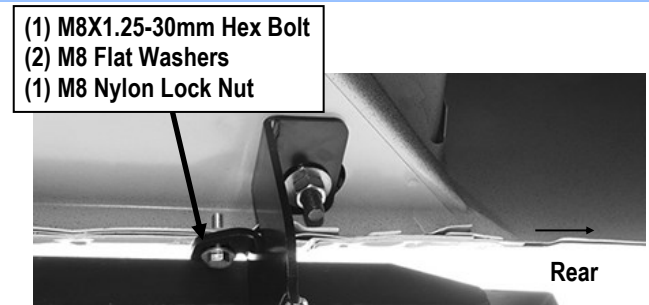
(Fig 19) Attach Passenger Rear Mounting Bracket (The Last One) to Pinch Weld
