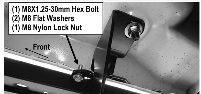
(Fig 17) Attach Passenger Center Mounting Bracket To Pinch Weld
