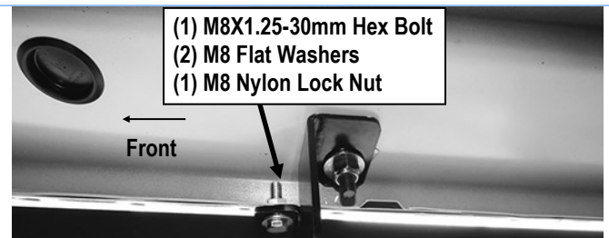
(Fig 18) Attach Passenger Rear Mounting Bracket (the 3rd one) to Pinch Weld
