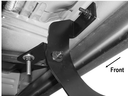
(Fig 9) Passenger Side Center Brackets Installed
