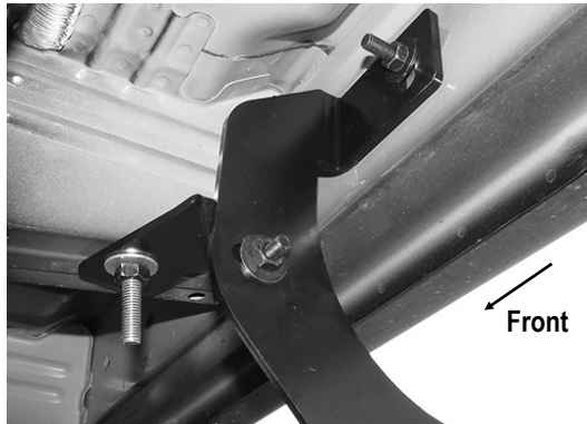
(Fig 9) Passenger Side Center Brackets Installed
