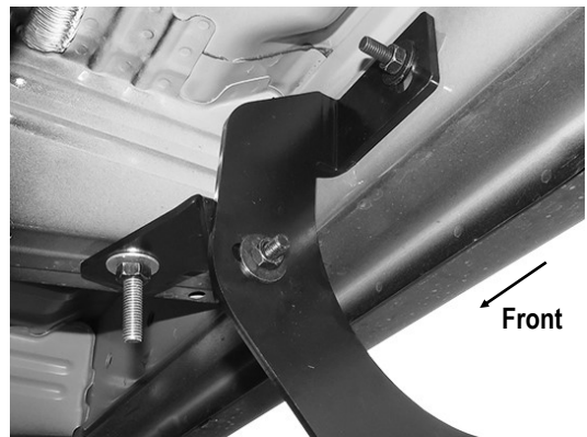
(Fig 9) Passenger Side Center Brackets Installed
