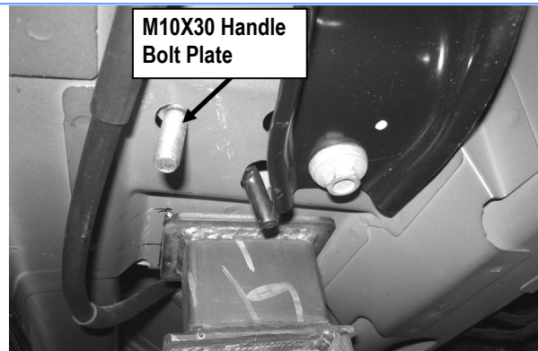
(Fig 5) M10X30 Handle Bolt Plate Installed
