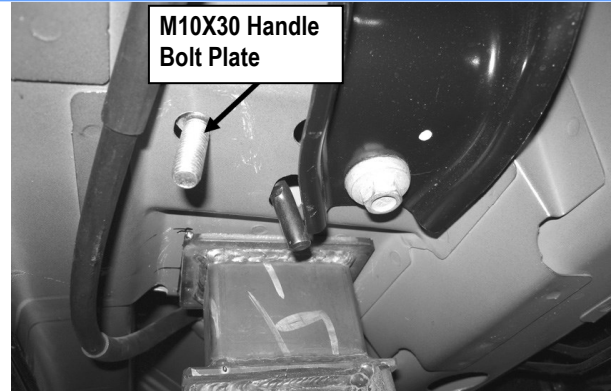
(Fig 5) M10X30 Handle Bolt Plate Installed
