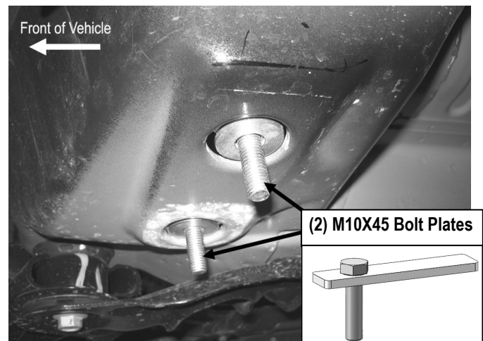
(Fig 1) M10X45 Bolt Plate Installation (Driver Side Front)
