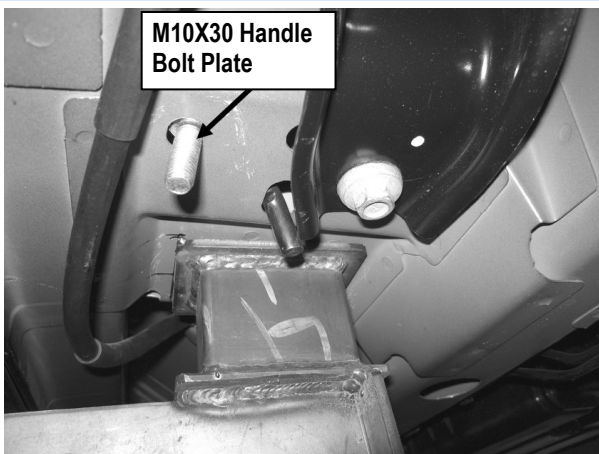
(Fig 6) M10X30 Handle Bolt Plate Installation
