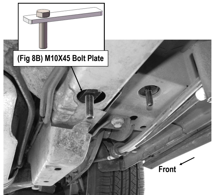
(Fig 8A) M10x45 Bolt Plate Installed (On Driver Side Rear Mounting Location)
