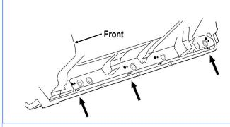
(Fig 1) Passenger Side Mounting Locations (Along Bottom And Inner Of the Body Panel)
