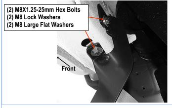
(Fig 6) Passenger Rear Mounting Bracket Installation
