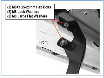
(Fig 4) Passenger Front Mounting Bracket Installation
