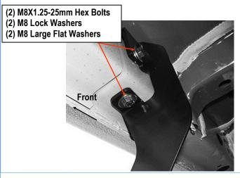
(Fig 5) Passenger Center Mounting Bracket Installation
