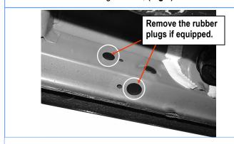
(Fig 2) Remove Plugs From Mounting Locations If Equipped
