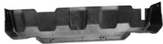
(Fig 14) 2017-Up Passenger Side DEF Cover Marked For Trimming
