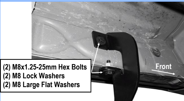
(Fig 5) Driver Front Mounting Bracket Assembly
