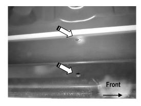
(Fig 5) Driver Side Rear Center Mounting Location
