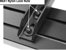
(Fig 9) Running Board Installed Onto Mounting Bracket
