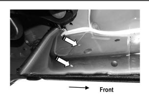
(Fig 6) Driver Side Rear Mounting Location
