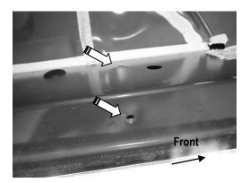
(Fig 3) Driver Side Front Mounting Location
