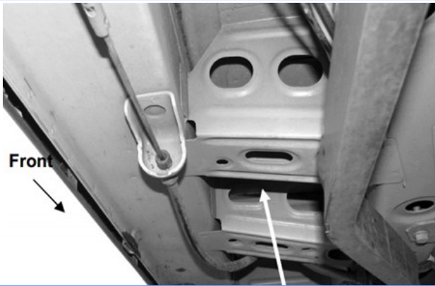
(Fig 5) Driver Side Center Mounting Location
