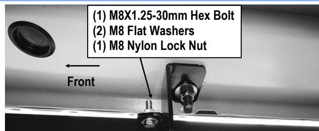
(Fig 20) Attach Passenger Rear Mounting Bracket (the 3rd one) to Pinch Weld
