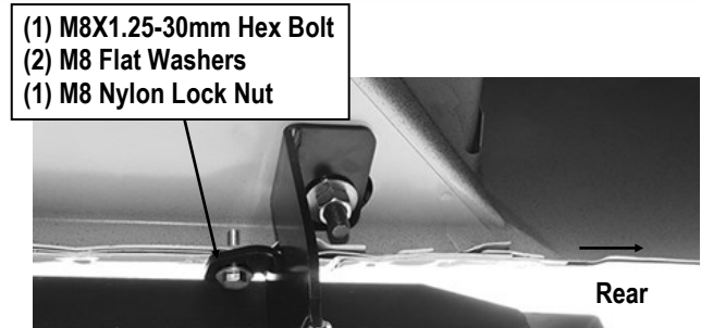
(Fig 21) Attach Passenger Rear Mounting Bracket (The Last One) to Pinch Weld
