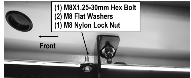
(Fig 20) Attach Passenger Rear Mounting Bracket To Pinch Weld
