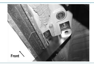
(Fig 3) Passenger Front Mounting Bracket Installed
