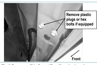
(Fig 4) Passenger Side Center/ Rear Mounting Location
