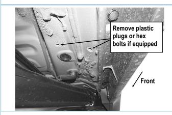
(Fig 1) Passenger Side Front Mounting Location
