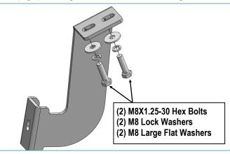
(Fig 5) Passenger Center/Rear Mounting Brackets Installation
