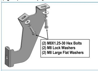
(Fig 2) Passenger Front Mounting Brackets Installation
