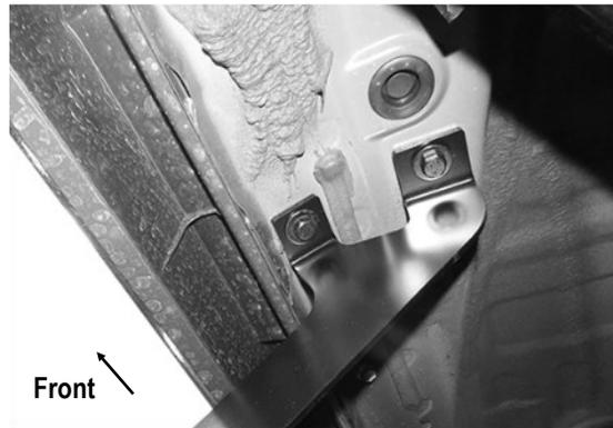
(Fig 3) Passenger Front Mounting Bracket Installed
