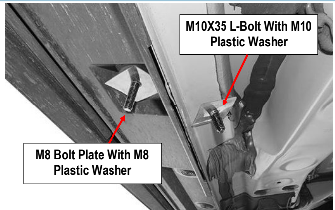
(Fig 13) M8 Bolt Plate & M10 L-Bolt Installed into Passenger Center Mounting Holes
