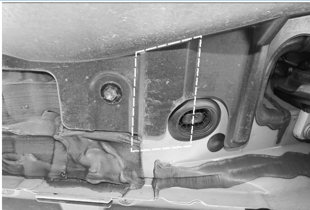
(Fig 7) Passenger Rear mounting location cut along dotted lines
