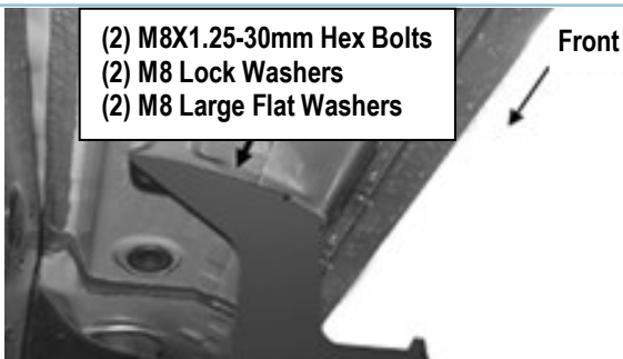
(Fig 2) Passenger Front Mounting Bracket Installation
