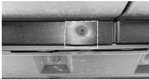
(Fig 5) Passenger Center mounting location (cut along dotted lines)
