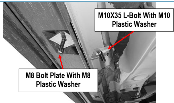
(Fig 14) M8 Bolt Plate & M10 L-Bolt Installed into Passenger Center Mounting Holes
