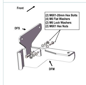
(Fig 4) Driver Front Mounting Bracket (DFM) And Driver Front Support Bracket (DFS) Assembly Pictured
