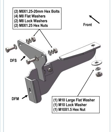
(Fig 5) The Assembled Driver Front Mounting Bracket Installation
