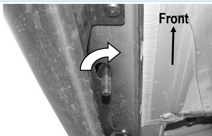
(Fig 3) Insert M10 Bolt Plate (Insert Bolt Plate then rotate 90-degrees or until it stopped for proper installation)
