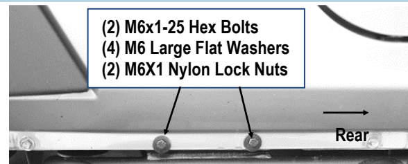
(Fig 10) Driver Front Support Bracket Installed
