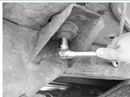
(Fig 1) Remove Factory Body Mount Bolt
