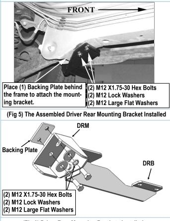
(Fig 6) Driver Rear Mounting Brackets Installation
