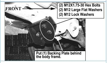
(Fig 2) Assembled Driver Front Mounting Bracket Installed
