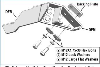
(Fig 3) Assembled Driver Front Mounting Bracket Installation
