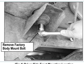
(Fig 1) Driver Side Front Mounting Location
