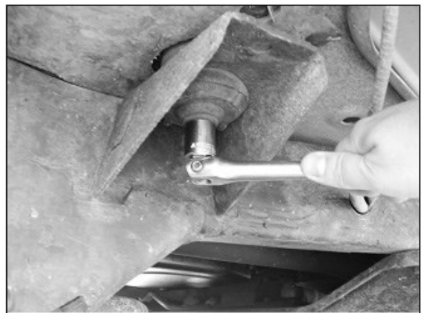
(Fig 1) Remove Factory Body Mount Bolt
