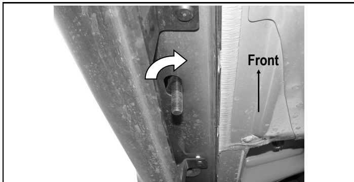
(Fig 3) Insert The M10 Bolt Plate
