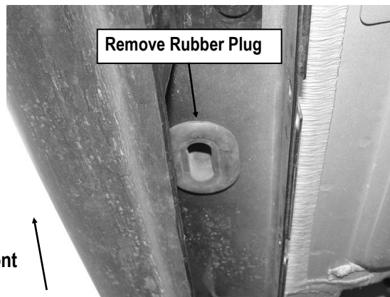
(Fig 2) Passenger Side Front Mounting Location on Rocker Panel
