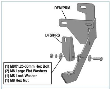
(Fig 1) Driver Side Front Brackets Assembly
