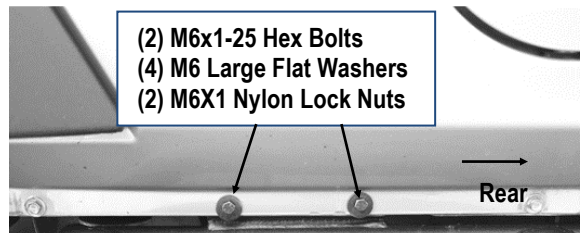
(Fig 10) Driver Front Support Bracket Installed
