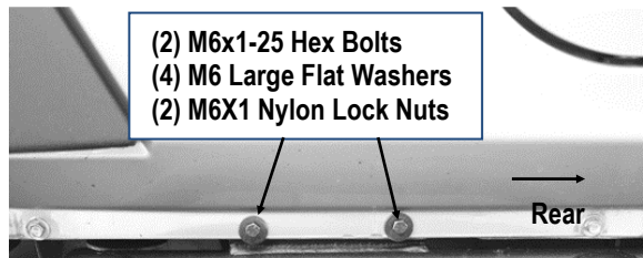
(Fig 10) Driver Front Support Bracket Installed
