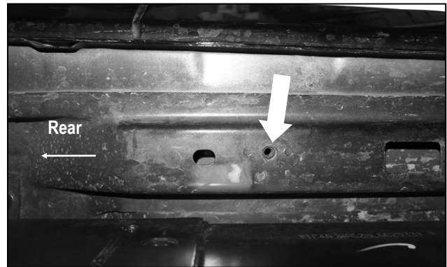
(Fig 5) Driver Side Center & Rear Mounting Location (Vehicles with factory threaded hole in floor panel)
