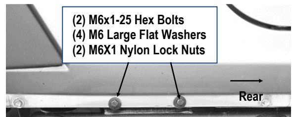
(Fig 10) Driver Front Support Bracket Installed
