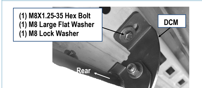
(Fig17) Driver Center Mounting Bracket Installed
