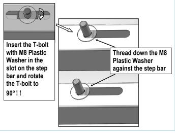
(Fig 8) T-Bolt with plastic washer in the slot
