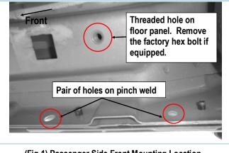
(Fig 1) Passenger Side Front Mounting Location
