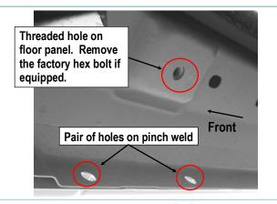
(Fig 2) Passenger Side Center Mounting Location
