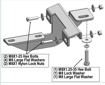
(Fig 4) Passenger Front Brackets Assembly
