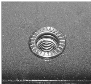
(Fig 8) Tighten Hex Bolt To Collapse And Lock Rivet Insert Into Factory Hole
