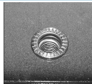
(Fig 10) Tighten Hex Bolt To Collapse And Lock Rivet Insert Into Factory Hole
