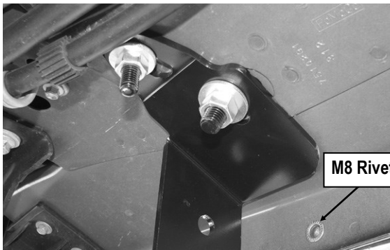
(Fig 14) M8 Rivet Nut Installed On Pinch Weld (Driver Rear Support Bracket Location)
