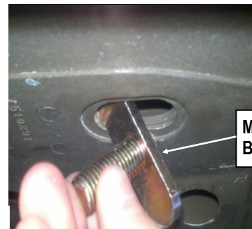
(Fig 4) Insert Bolt Plate Into The Front Driver Side Slot Under The Vehicle
