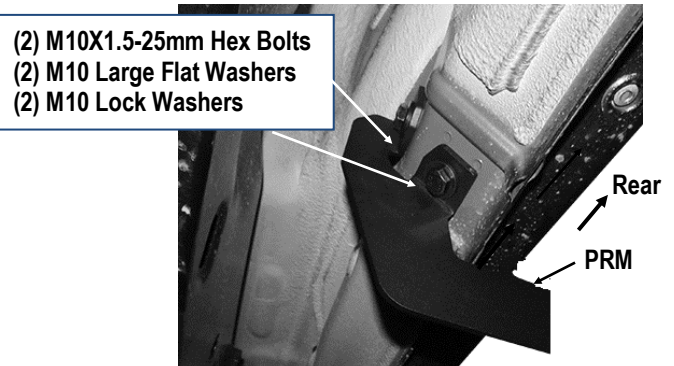
(Fig 7) Passenger Rear Mounting Bracket Installed
